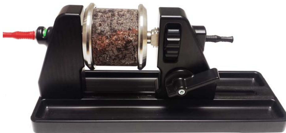
IP-T10 Reference Pad with Sample Holder
