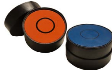
Magnetic Susceptibility Calibration Pads
