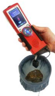
Density Measurement: Sample Submerged in Water
