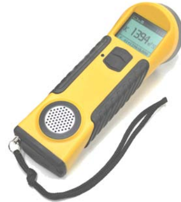
KT-10 v2 Magnetic Susceptibility Meter (Circular Coil)
